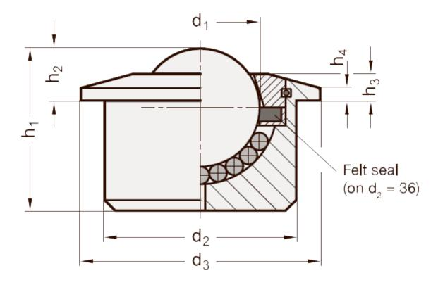
$$\begin{array}{lll} d1 & = 44.4 \\ d2 + / -0.08 & = 62 \\ d3 & = 75 \\ h1 + / -0.3 & = 53.5 \\ h2 + / -0.3 & = 19 \\ h3 + / -0.3 & = 9.5 \\ h4 & = 5.5 \\ Max load (N) = 4500 \\ \end{array}$$
